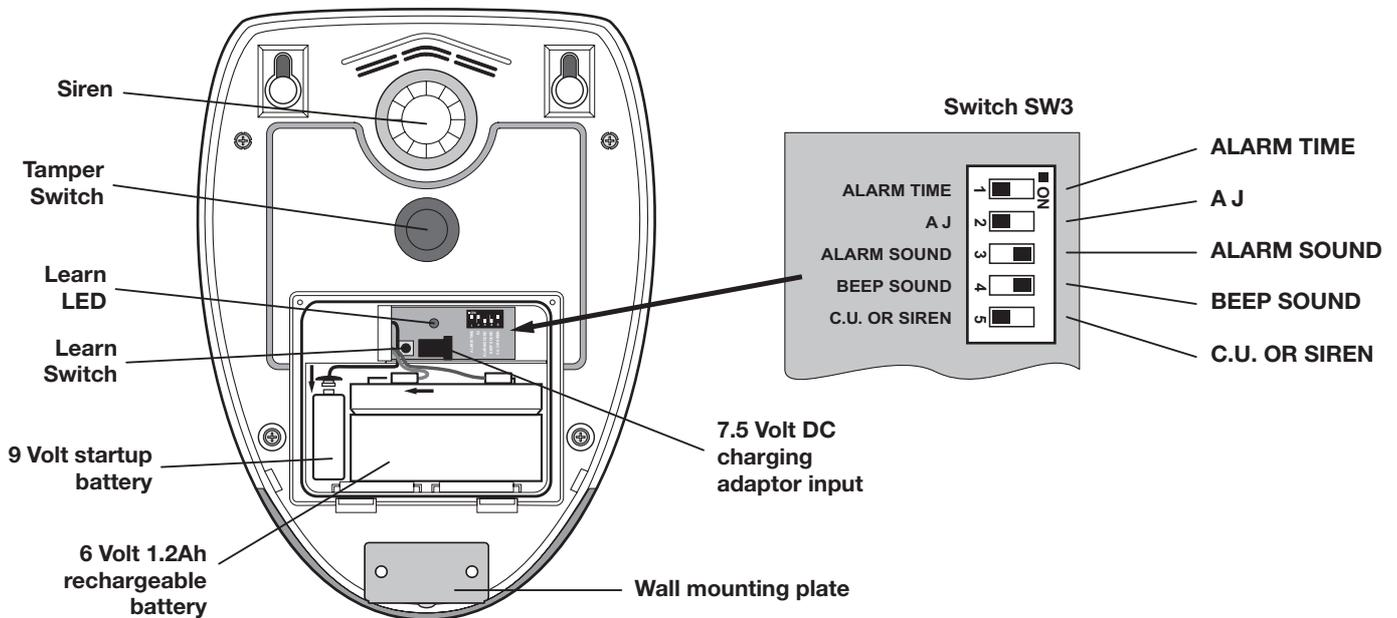
5. DIP switch 2 marked “AJ” does not function for this system and should be ignored.
