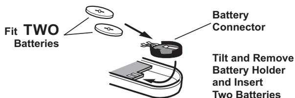
3. If necessary, refit the battery holder into the detector ensuring that the spring clip connectors slide onto either side of the circuit board.
