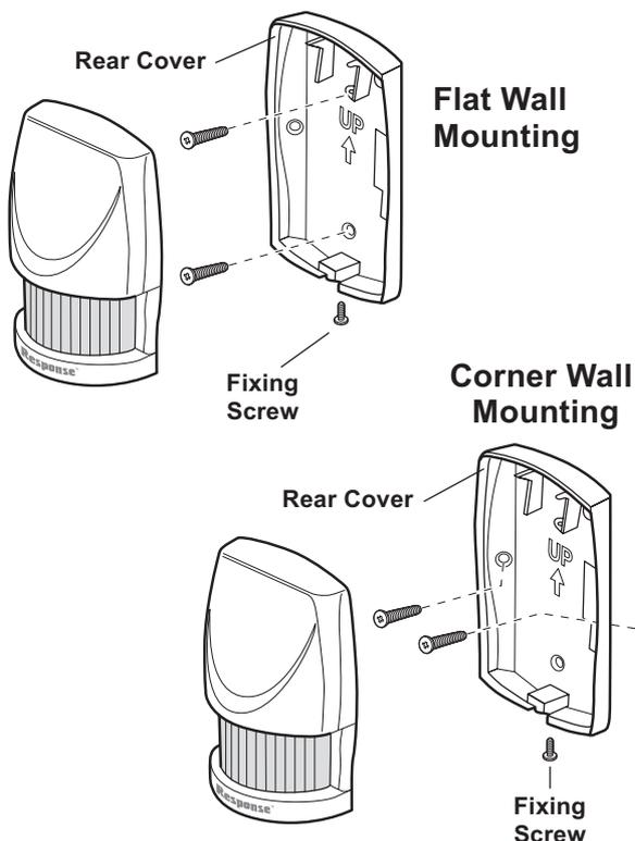
1. Undo and remove the fixing screw from the bottom edge of the PIR Detector, (keep the screw safe for later). Carefully pull the bottom edge of the detector away from the rear cover and then slide down to release the top clips.
