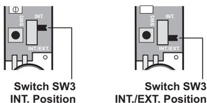
If setting to the INT. position, only the internal contact will be active. When two contacts are in use for internal and external connection simultaneously (INT./EXT. position), only one activation will be counted if one of the contacts is opened. If one contact is left open and the other closed contact is opened then an activation will be counted.
