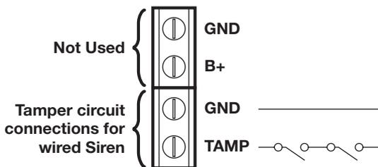
The Control Panel incorporates a terminal block for connection of a Hard-wired Siren. The connection terminal block is located inside the Control Panel behind the front cover. To access the terminal block
