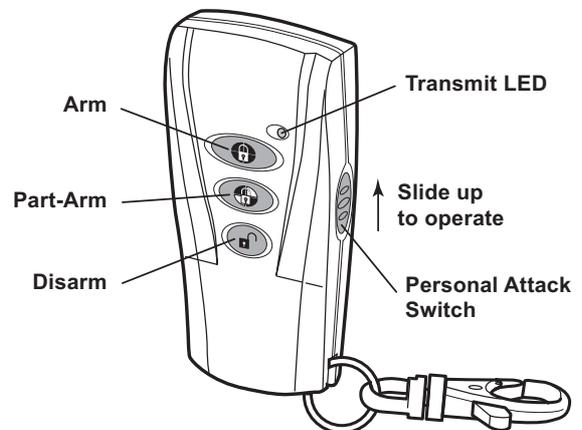
The Remote Control Unit also incorporates a Personal Attack (PA) switch. Activating the PA switch on the side of the Remote Control will immediately trigger an Alarm (unless the Control Panel is in Test or Program Modes) even if the system is disarmed. The alarm can be cancelled using the Remote Control by pressing the 'DISARM' button.
